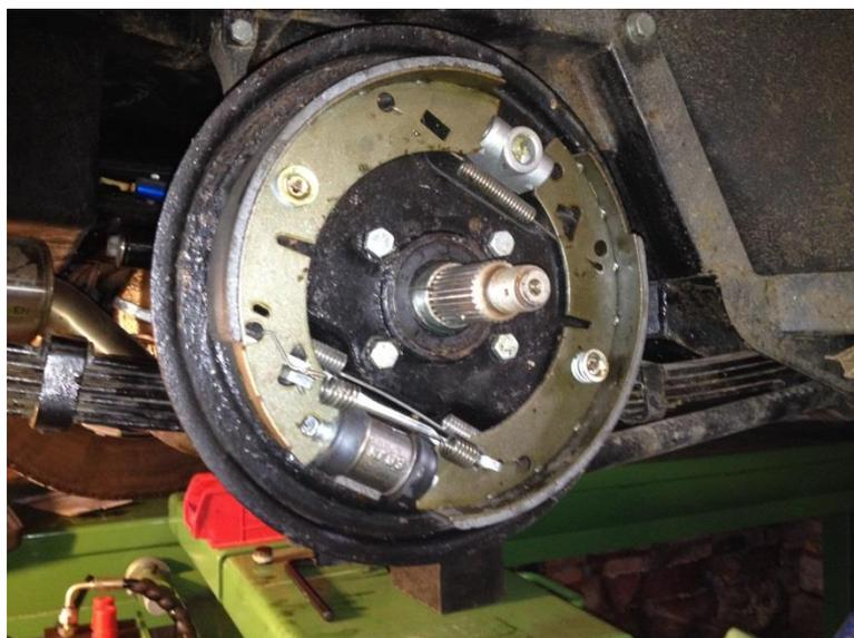
As previously mentioned, I also replaced the brake shoes as I'd had an oil leak.
