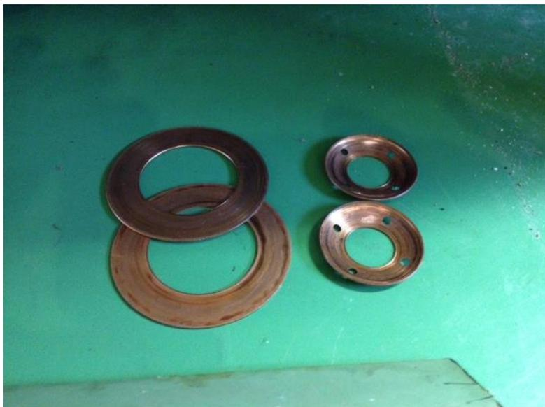
The larger phenolic washers are under the side spur gears and the cupped washers are under the top and bottom planetary gears. Smear the new spacer washers in new diff oil, refit the side spur gears with the phenolic spacers fitted and roll the top and bottom planetary gears, with new cupped washers, back into place. This is a little fiddley as the new washers
