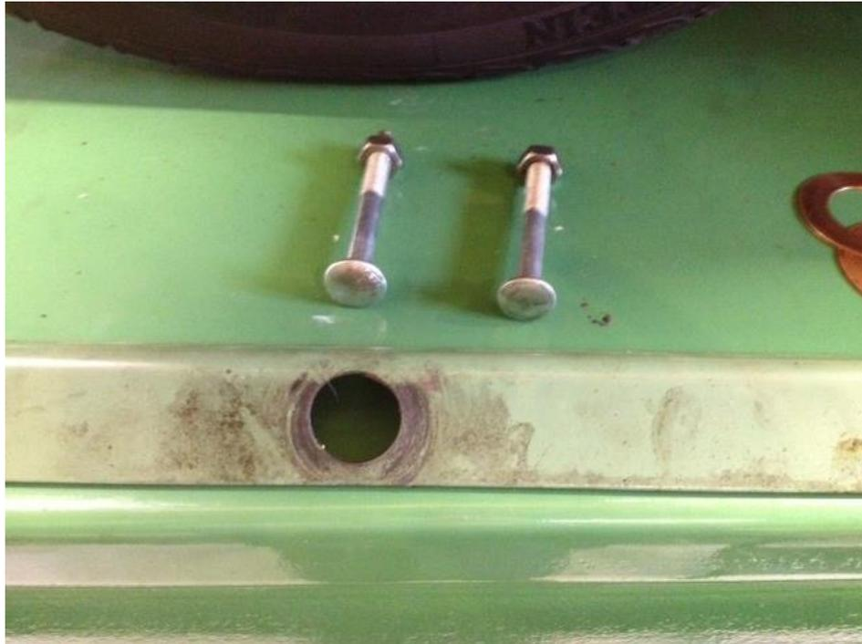
The half shaft pokes through the hole and the coach bolts sit in the holes in the end of the axle case where the back plate bolts to with the heads up against the angle and the using the hub nut on the end of the half shaft wind this in and it pulls the half shaft out. You will have to wind the nuts down the coach bolts to space the angle further out when the hub nut bottoms out on the half shaft.
