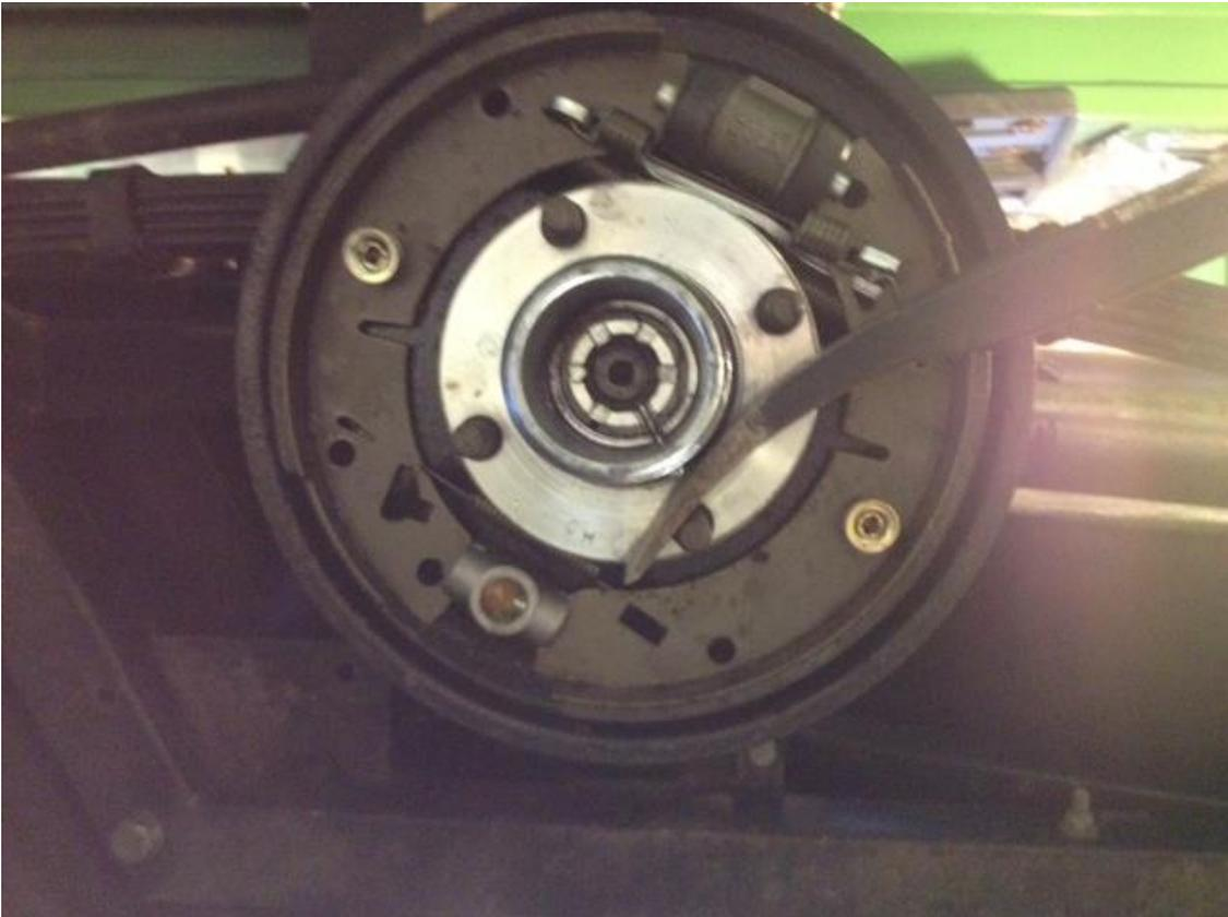
Once the hub is off, disconnect the brake pipe from the slave cylinder and plug the pipe (I used a spare slave cylinder) to stop you losing all of the brake fluid, disconnect the handbrake cable and remove the brake back plate and the last item, the bearing cover plate.
