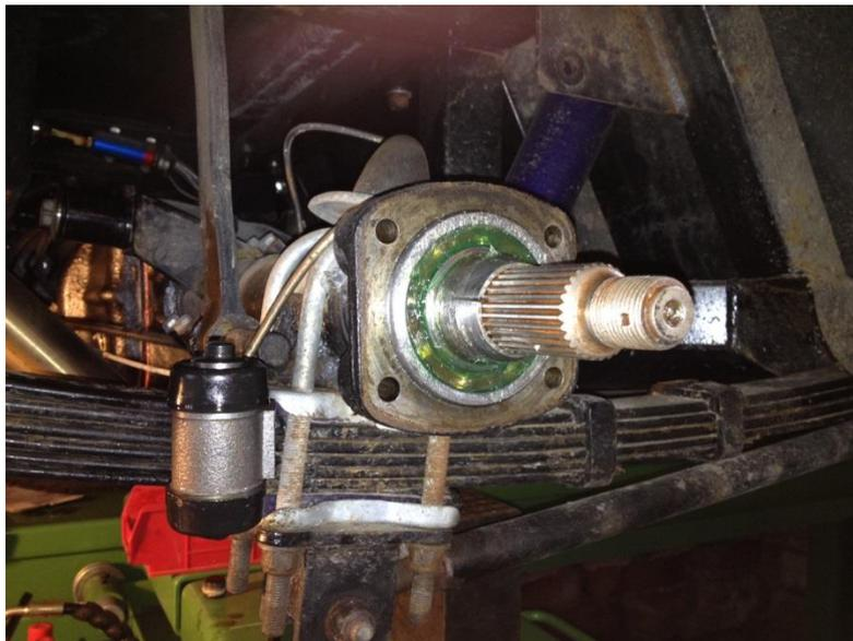
I replaced the oil seal and collar that it runs on as they were also worn. Ensure that the inner lip of the oil seal is also greased. The back plate can now be refitted, brake pipe can be connected to the slave cylinder and handbrake cable can be reconnected.
