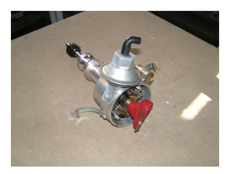
Lever off the rotor arm with a screwdriver. I found it best to use a large screwdriver between the base of the rotor arm and the points cam and twist the screwdriver to lever it off.
