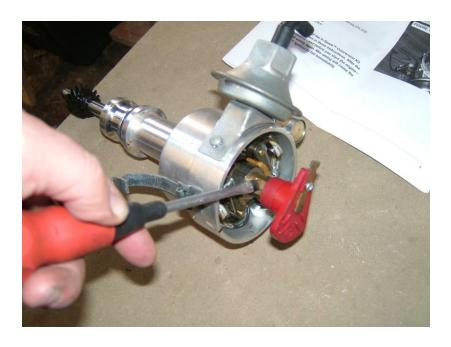
Next up is to remove the condenser bracket, insulators, e clip that holds the vacuum advance arm to the points plate and vacuum advance canister. These bits are explained really well in the instructions hence the reason why I've
